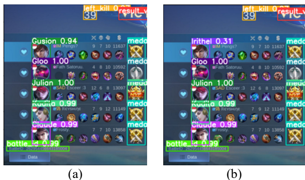
Figure 5. Example of multiple overlapping detection on one object: (a) correct prediction on top, (b) wrong prediction on top
