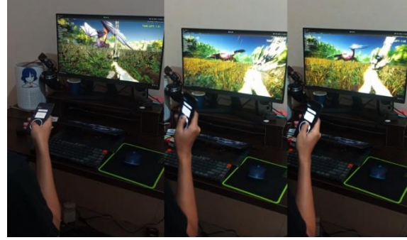
Fig. 10 Alternating sword by swinging wireless mobile phone with gyroscope.
