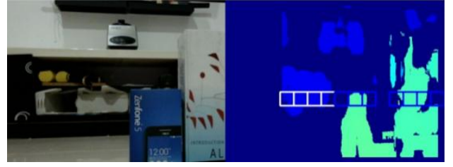
Figure 4. Obstacle Detection Sample: (Top-Left) Right Maneuver Scenario Where Obstacle is in Left, (Top-Right) Left Maneuver Scenario Where Obstacle is in Right, (Bottom) Stop Scenario Where Obstacle is too Close to Robot
