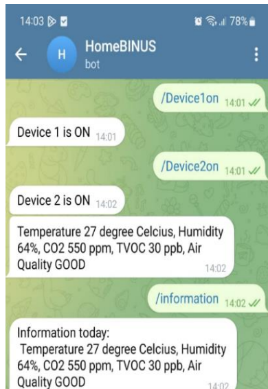
Fig. 9. Using Telegram, we can control devices and get information from the sensors.
