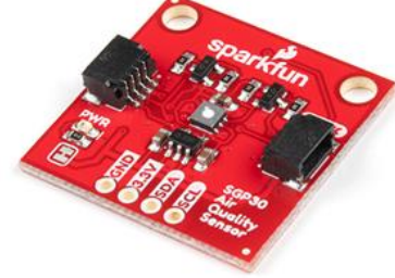
Figure 5. Module of Air quality sensor SGP30, with type of Qwiic [6].
