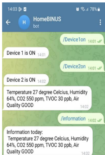
Fig. 9. Using Telegram, we can control devices and get information from the sensors.
