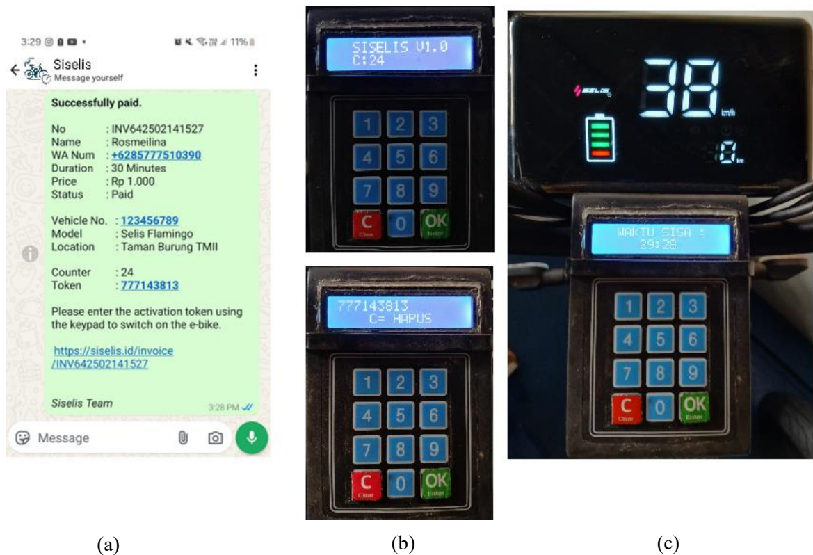
Fig. A3. Implementation of the system: (a) message containing the digital receipt and activation token, (b) e-bike rental interface in standby status, (c) e-bike rental interface in active status with the e-bike powered up. Note: hapus means delete, and waktu sisa is remaining time.
