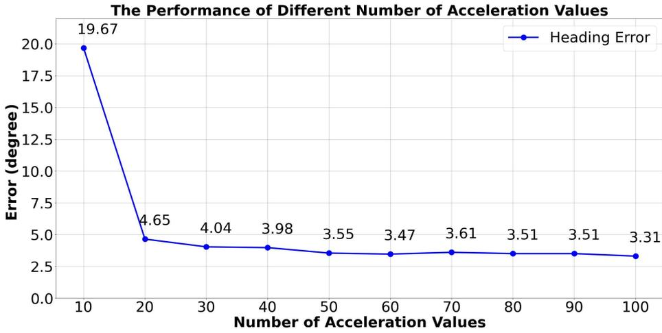
Fig. 6. The heading errors when using a different number of acceleration values for the Principal Component Analysis (PCA) method.
