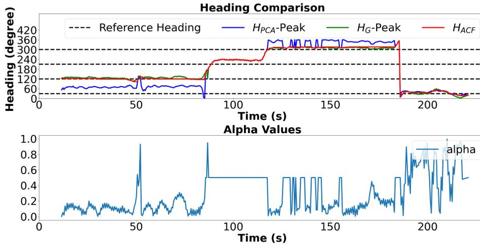
Fig. 12. Heading Errors of swinging the phone freely along the pedestrian’s walking direction (SW) in the second walking path among three methods.
