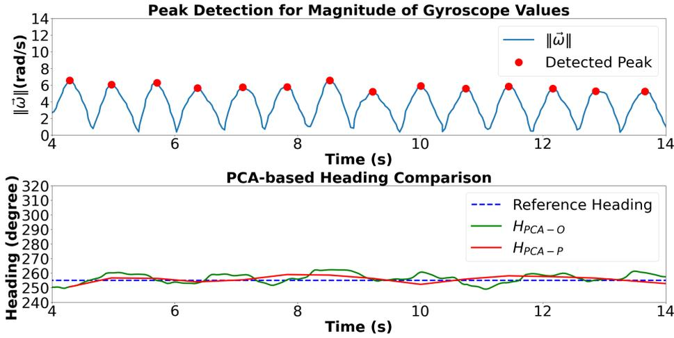
Fig. 5. The difference in heading estimation between two Principal Component Analysis (PCA)-based methods.
