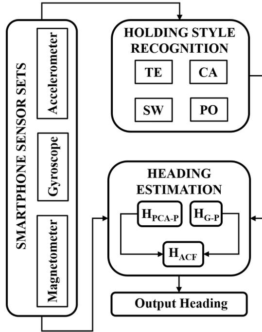
Fig. 1. Overview of the proposed method. It consists of holding the smartphone in front of the pedestrian’s body for reading or texting (TE), holding the smartphone against the ears for making a phone call (CA), swinging the phone freely along the pedestrian’s walking direction (SW), and putting the phone into the pants’ front pockets (PO), PCA-based heading  $H_{PCA-P}$ , gyroscope-based heading  $H_{G-P}$ , and the proposed adaptive heading  $H_{ACF}$ .
