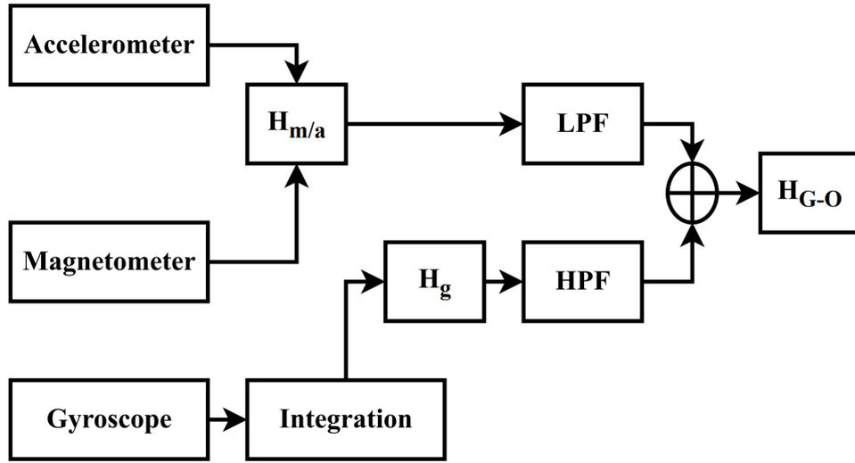
Fig. 7. The diagram of the gyroscope-based heading estimation method. Absolute heading calculated from the accelerometer and the magnetometer ( $H_{m/a}$ ), relative heading calculated from the gyroscope ( $H_g$ ), heading calculated from  $H_{m/a}$  and  $H_g$  using the complementary filter ( $H_{G-O}$ ), Low-Pass Filter (LPF), and High-Pass Filter (HPF).
