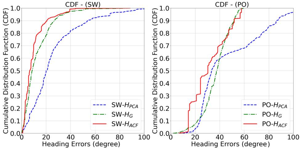
Fig. 11. Cumulative heading error distributions of swinging the phone freely along the pedestrian’s walking direction (SW) and putting the phone into the pants’ front pockets (PO) in the first walking path.
