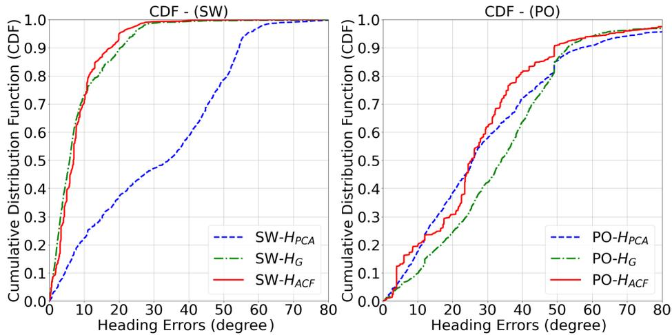
Fig. 13. Cumulative heading error distributions of swinging the phone freely along the pedestrian’s walking direction (SW) and putting the phone into the pants’ front pockets (PO) in the second walking path.
