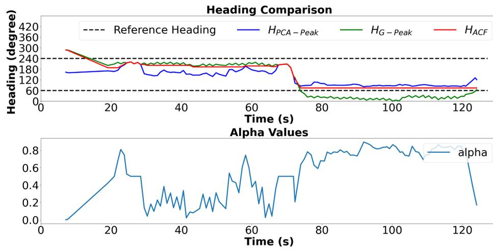
Fig. 10. Heading errors of putting the phone into the pants’ front pockets (PO) in the first walking path among three methods.
