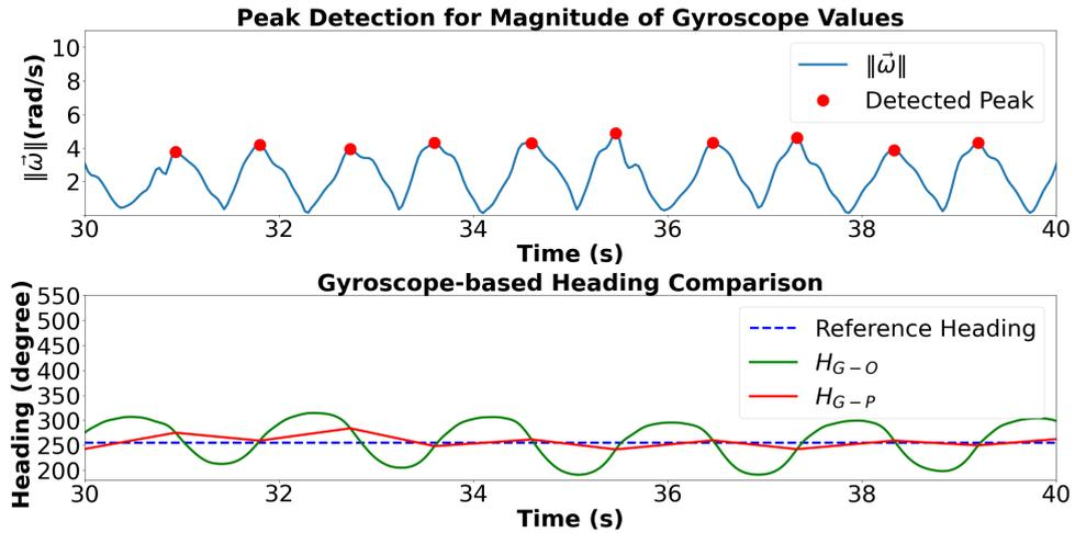
Fig. 8. The difference in heading estimation between two gyroscope-based methods.
