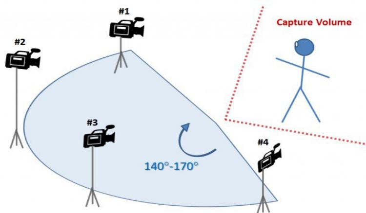
**Figure 2.** We use four-camera setup to capture the movement
